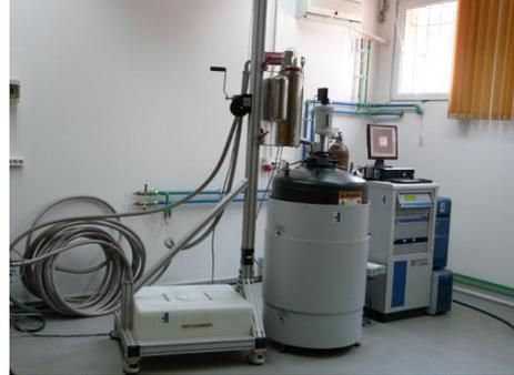
Different Magnetic Properties Measurement Systems, such as vibrating sample magnetometer or SQUID allow research on magnetic materials, spintronics and superconductors.
