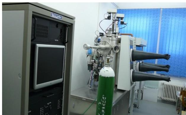
A wide range of preparation techniques is available, permanently new materials being created by the Institutes research teams. Thin films ranging from transparent conducting oxides, organic semiconductors or ceramics to magnetic metals are prepared by physical deposition methods such as Pulsed Laser Deposition, vacuum evaporation or magnetron sputtering.
